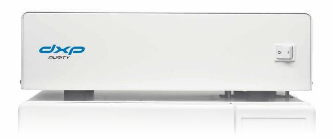
Compliant with the EN 1717 standard, DXP Purity is a special fully automatic reverse osmosis system with three filters, to be placed on top of the autoclave to connect it to the mains water system and produce between 1,000 and 2,000 litres of high-quality demineralised water. Depending on the consumption of the autoclave, this makes it possible to carry out between 2,000 and 4,000 sterilization cycles effectively and reliably.
